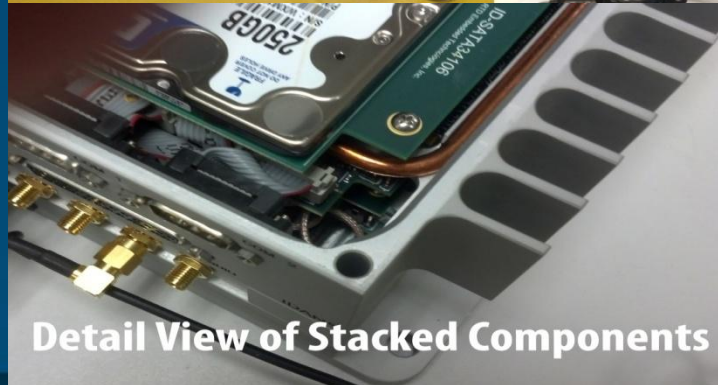
CoE prototype PC/104 board stack in a hardened case The visible board is a single-board computer with a 250GB hard-disc drive. Sitting below, in the stack, are other interconnected PC/104 compatible development boards and a power supply
